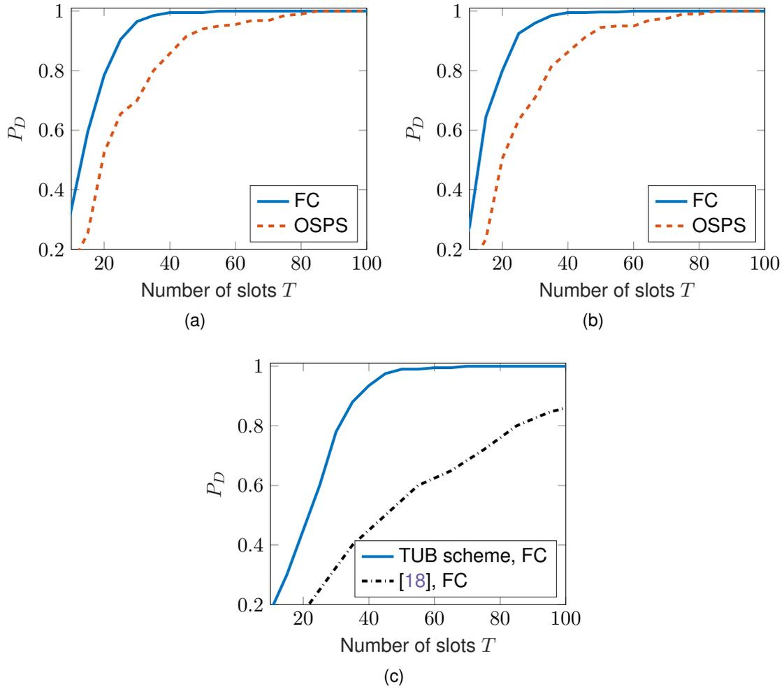
Figure 3.4: Detection probability  $P_D$  of different transmitter architectures vs. the training overhead for the initial beam alignment phase with (a)  $\text{SNR}_{\text{BBF}} = -20$  dB, (b)  $\text{SNR}_{\text{BBF}} = -5$  dB, and (c) a comparison with the literature.
