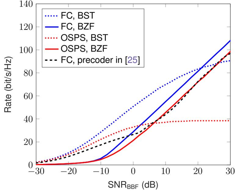
Figure 4.1: The sum spectral efficiency of both architectures vs. increasing  $\text{SNR}_{\text{BBF}}$  for the data communication phase with different precoding schemes.
