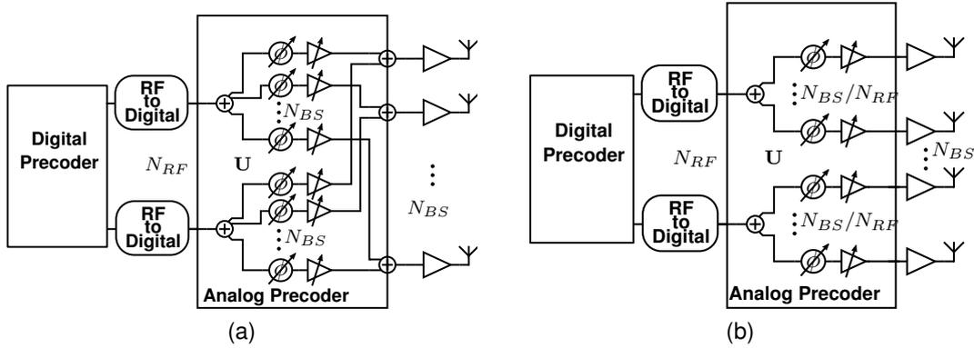
Figure 2.1: Hybrid transmitter architectures: (a) fully-connected (FC), and (b) one-stream-per-subarray (OSPS).
