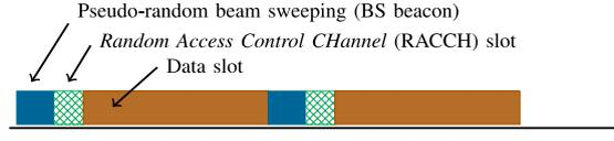
Figure 3.2: Diagram of the frame structure.
