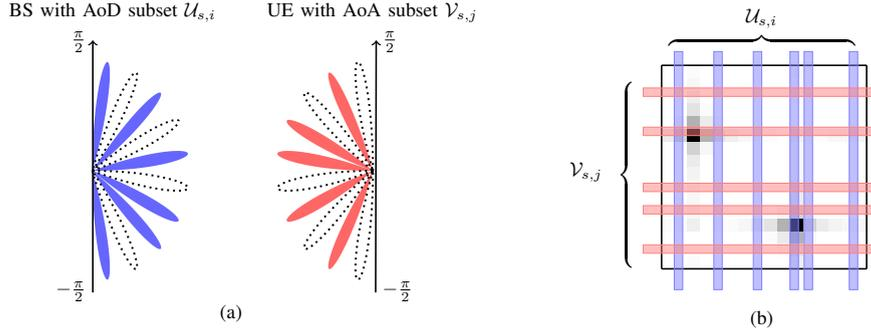
Figure 3.3: Illustrations of the beamforming codebooks for one beacon slot: (a) the beam patterns of the base station and a UE and (b) the channel with two strong paths (indicated by dark spots) probed with the beam patterns.
