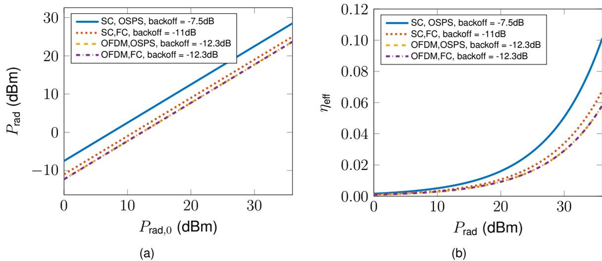
Figure 2.2: The power efficiency evaluation of both architectures in terms of (a) the actual radiated power in *option I* vs. the radiated power of the reference scenario, and (b) the power efficiency in *option II* vs. the actual radiated power.
