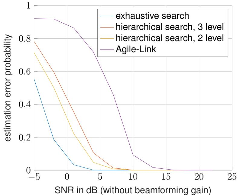
Figure 3.1: Measured average probability of error estimating the AoA for the basic BA algorithms.
