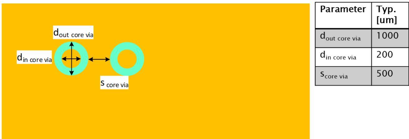
Figure 5: Sketch of copper core vias (top view) with design rules
