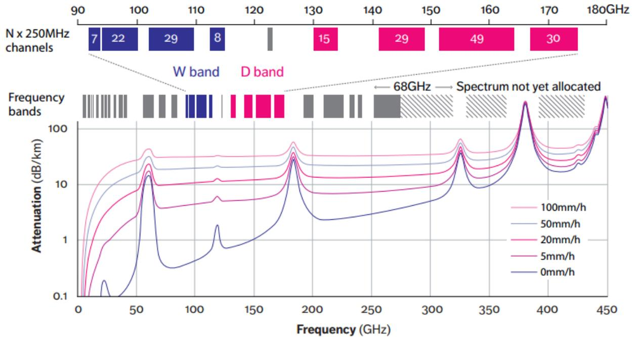
Figure 2: Atmospheric attenuation beyond 100 GHz
